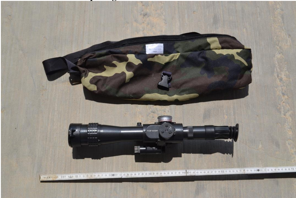
Figure 20.36 POSP 12x50M Telescopic Sight manufactured in Belarus
