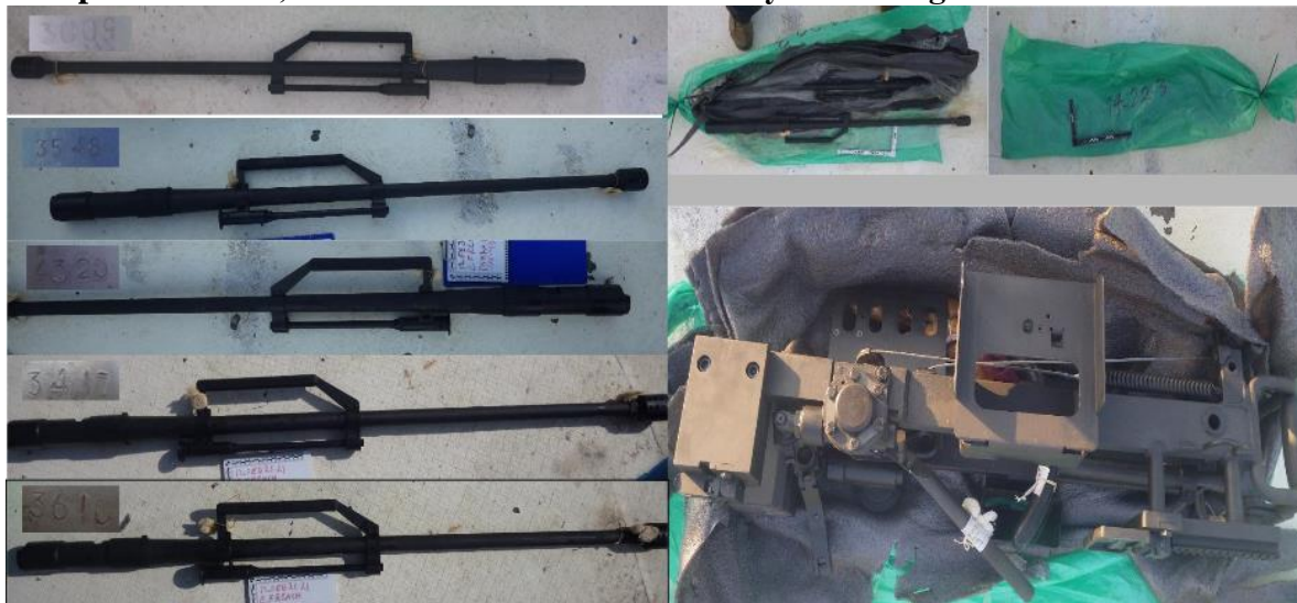
Figure 19.12 Components of 12,7x108mm calibre 'DSchK' heavy machine guns
